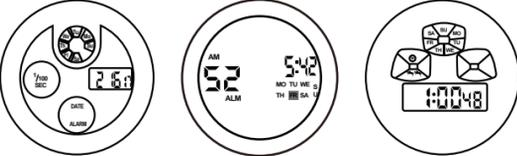
Under standard time display mode, press Key C+D to switch on / off alarm.
